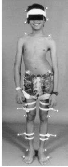
Figure 9: The marker configuration by Masso and Gorton [19]
